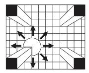
The 270 Degree dome serves the same purpose as the full dome except it is not centrally located in an intersection. Usually when a 270 Degree dome is used, it is in an area with narrow aisles or in a lobby of a building.
