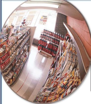
Convex mirrors should be mounted at the end of alternating aisles to reflect the view of the traffic moving from the neighboring isles. Small convexes can be used in offices to view hallways or reception areas for visitors
