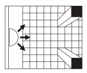
For industrial use larger domes can be mounted on the end of aisles at a lower level than most full domes. These half domes would be mounted at the end of an aisle where a forklift operator can see in both directions without needing to look towards the ceiling. Hardware Included.
